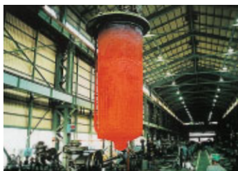
Titanium Sponge Manufacturing (Toho Titanium Co., Ltd.)
