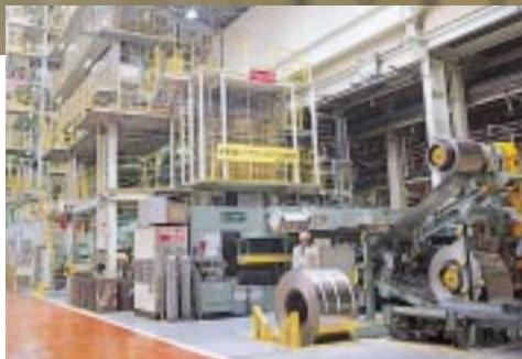
Continuous Bright Annealing Line, Kurami Works
