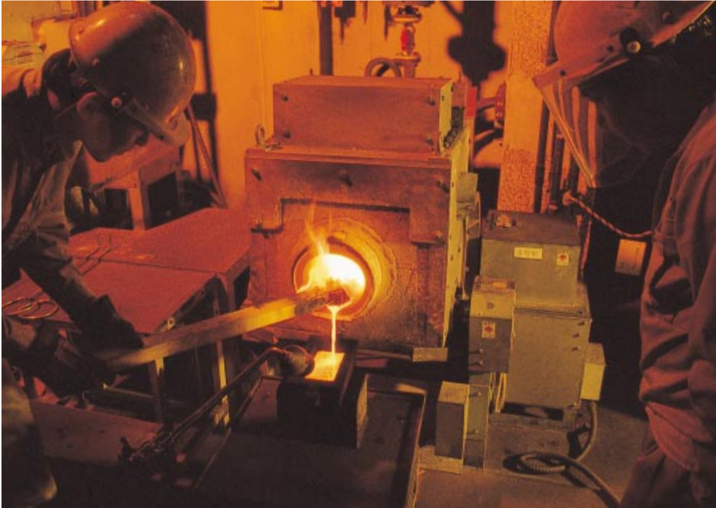
Gold Casting Operations, Saganoseki Smelter & Refinery
