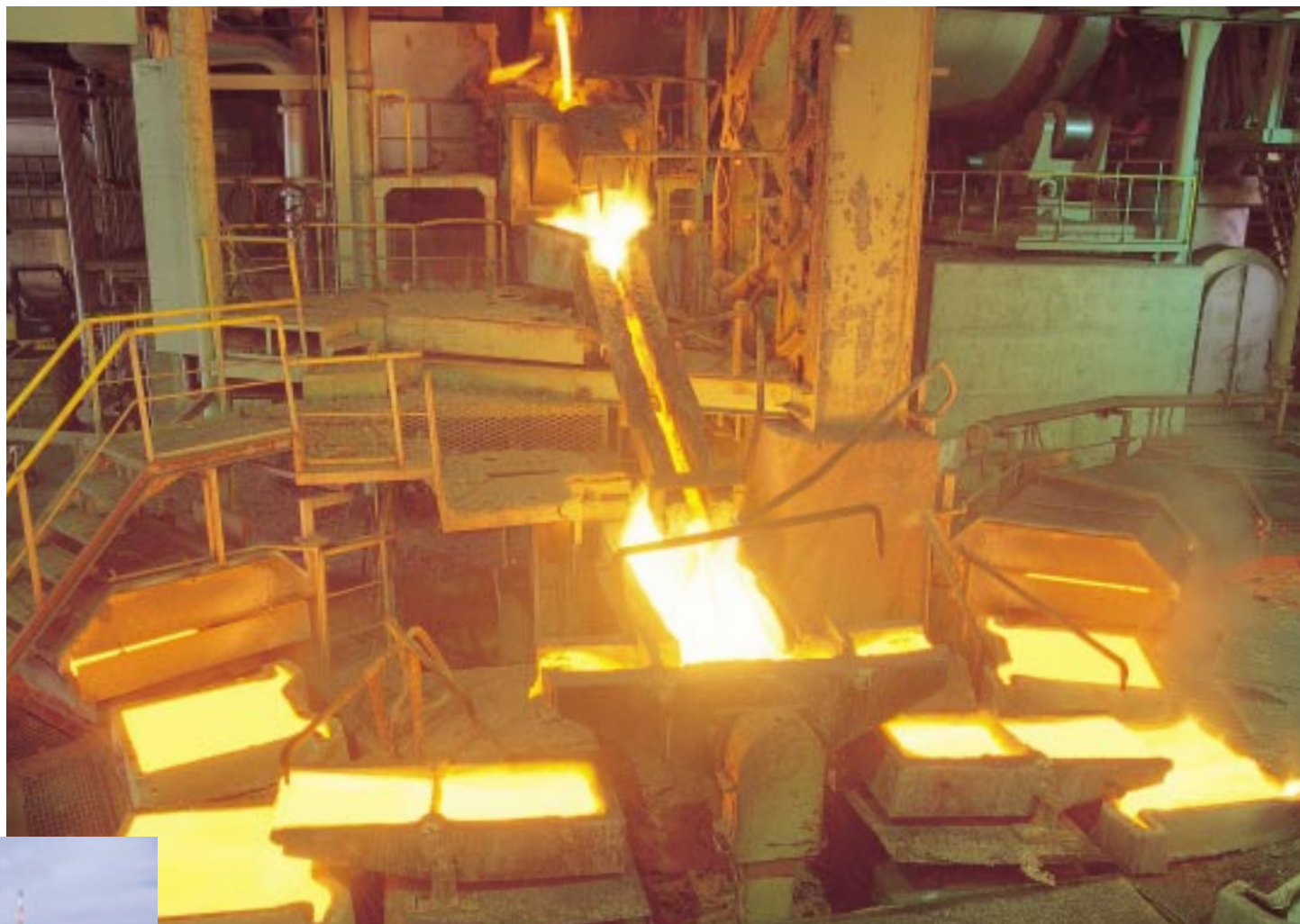
Anode Furnace and Anode Casting Wheels, Saganoseki Smelter & Refinery
