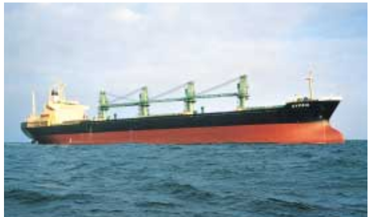
“Cypria,” a dual-purpose carrier that ships sulfuric acid and copper concentrate
